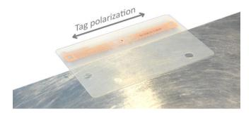
Select the location carefully in a vehicle body, as good placement will ensure smooth identification in every stage of manufacturing until the end of assembly line and beyond.
