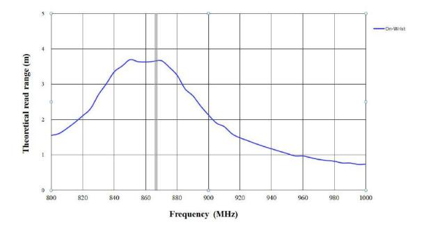
Reading distance might differ on the material which the tag is attached. SAG can help fine tune the antenna to obtain the optimized reading performance.
