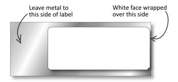
Smallest recommended bending diameter of the Confidex ESD On Metal Label™ is 100mm. For optimal performance please bend the label in the orientation shown below.
